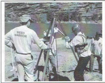
The 'pod squad' then moved in with the real muscle on the trip: a tripod made of 2 inch square tube steel about 7 ft tall. Hanging from the top of the tripod was a
